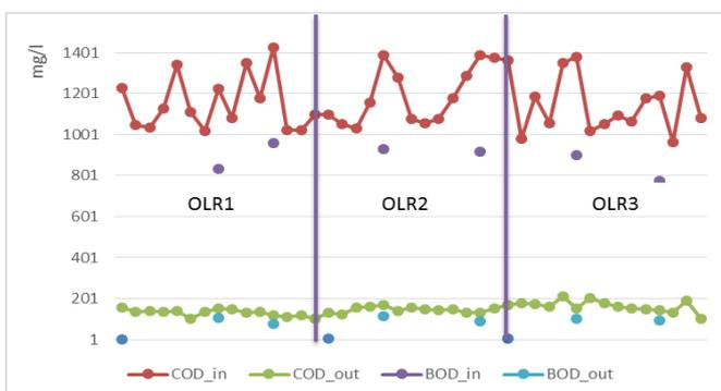
The model was operated continuously for 120 days (including 30 days for startup), one loading rate each month, from 1.5 to 6.5 kg COD/m<sup>3</sup>/d.
