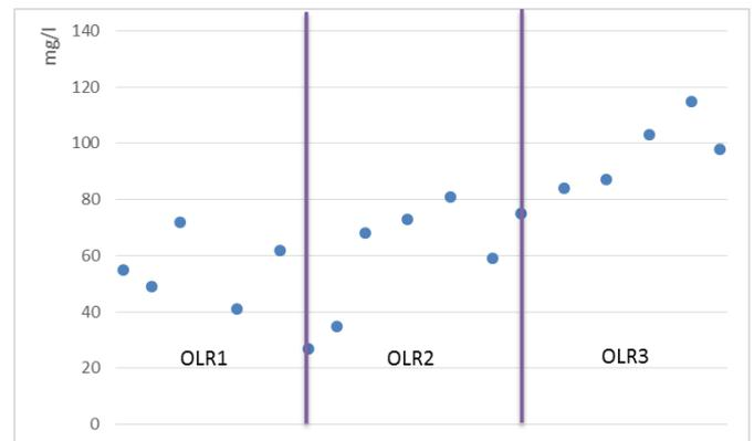
**Fig. 4. The changes in SS outlet through 3 OLRs**
