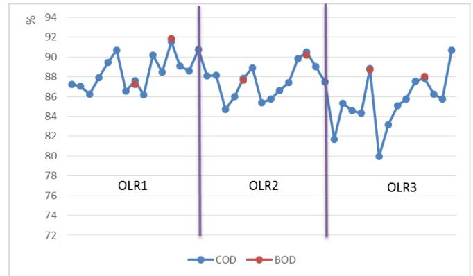
**Fig. 3. The changes in COD, BOD efficiency through 3 OLRs**
