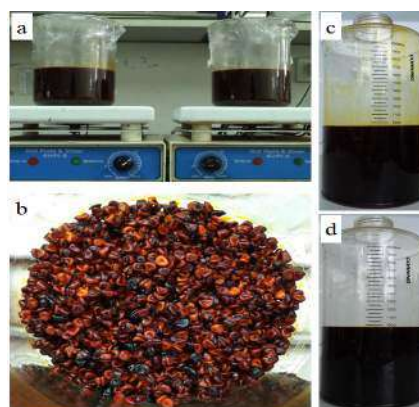
Fig 1. Extracting and converting process into norbixin (a: stirring process, b: waste matter, c: extractive solvent was filtered, d: extractive solvent was incubated)
